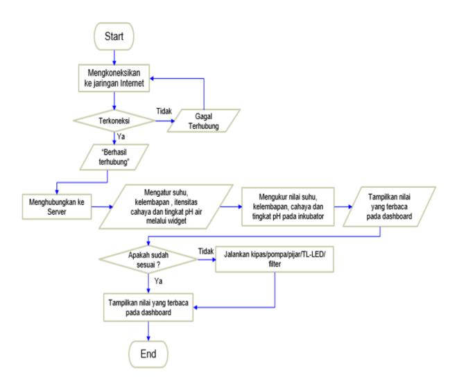
Gambar 3.10 Flowchart Sistem Inkubator
