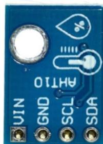
Gambar 3.3 Sensor AHT10 [17]
